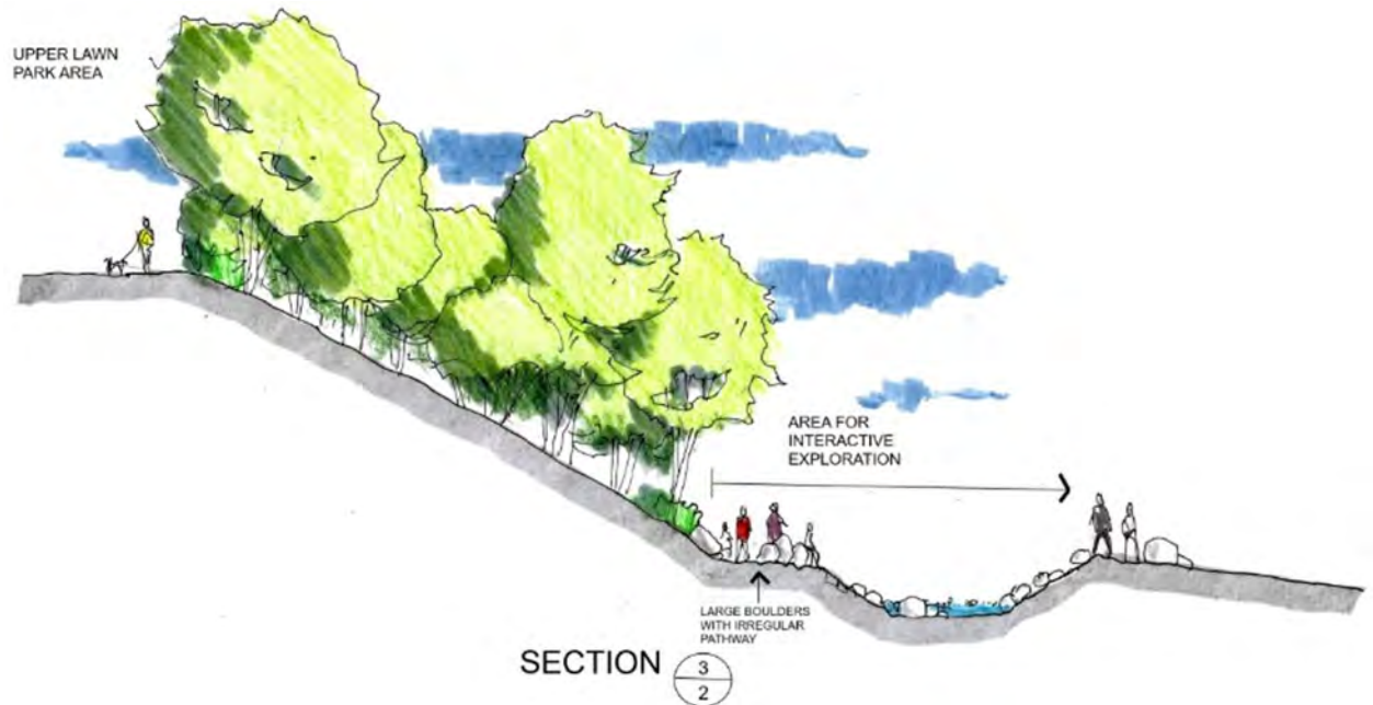
Figure 8. Conceptual section view of the Montgomery Dam dam removal case with restored channel alignment.
