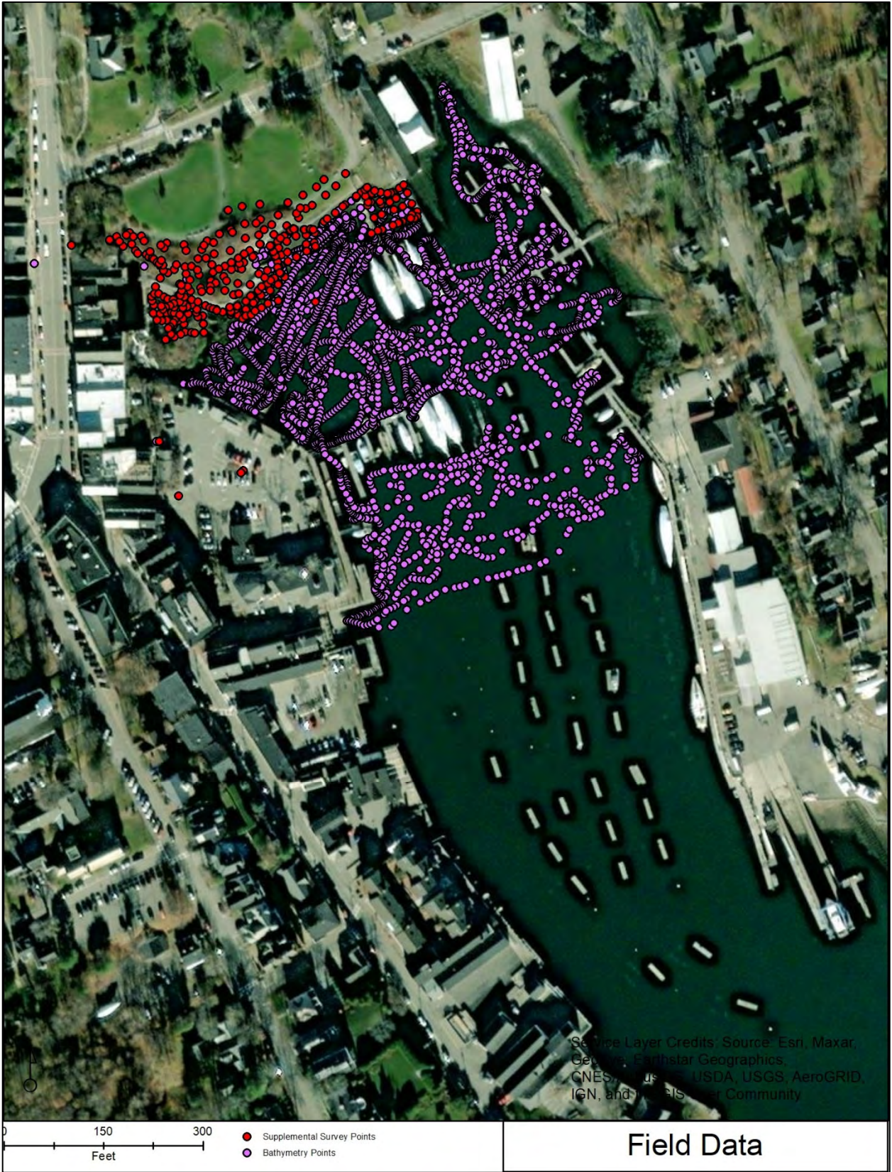
Figure 1. Distribution of bathymetric and supplemental terrain survey points.
