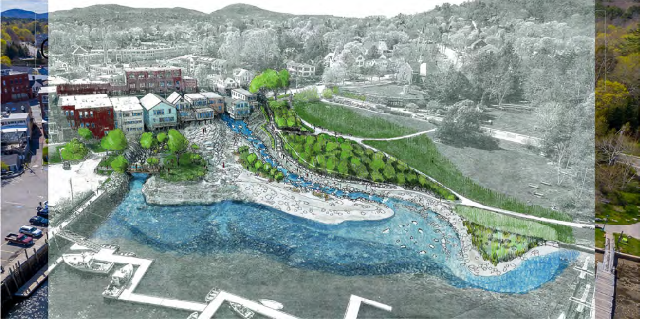
Figure 5. Conceptual rendering of the Montgomery Dam dam removal case with restored channel alignment at low river flow and mean tide level.
